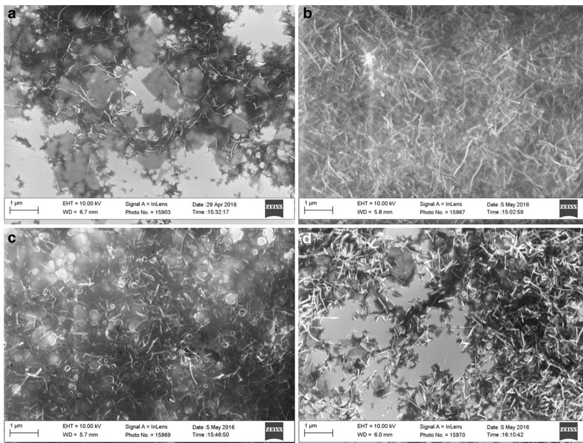
**Fig. 6** Scanning electron microscopy (SEM) micrographs of TeNRs<sub>100</sub> (a), and TeNRs<sub>500</sub> (b) produced by *unconditioned* BCP1 K<sub>2</sub>TeO<sub>3</sub>-grown cells, and TeNRs<sub>100</sub> (c), and TeNRs<sub>500</sub> (d) extracted from those *conditioned*
