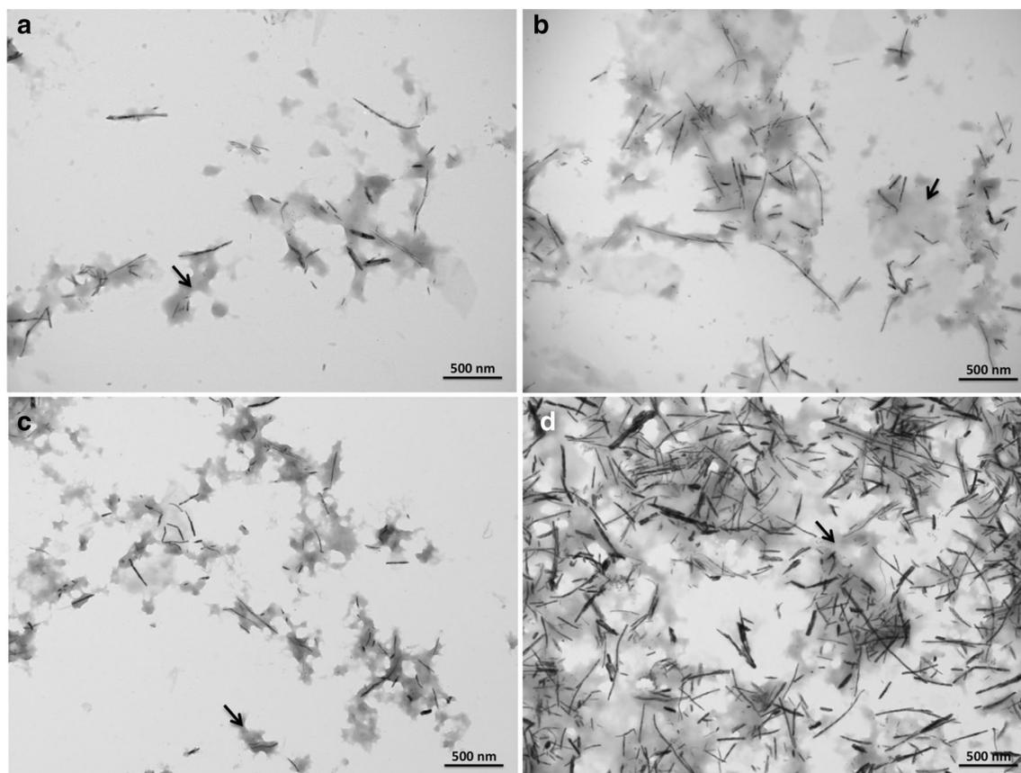
**Fig. 4** Transmission electron microscopy (TEM) micrographs of TeNRs<sub>100</sub> (a), and TeNRs<sub>500</sub> (b) extracted from the BCP1 strain grown as *unconditioned* cells in the presence of K<sub>2</sub>TeO<sub>3</sub>, and TeNRs<sub>100</sub> (c), and TeNRs<sub>500</sub> (d) recovered from those *conditioned*
