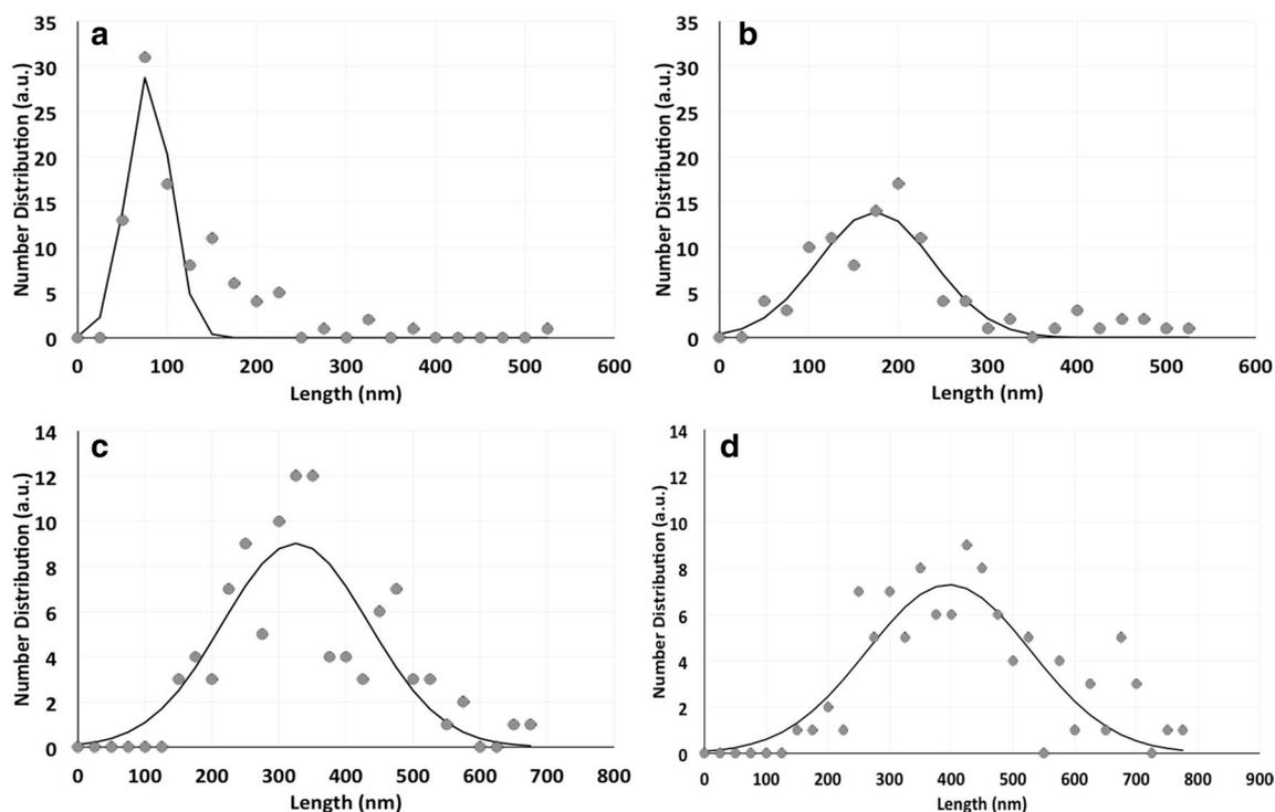
**Fig. 5** Length distribution (nm) of TeNR<sub>100</sub> (a), and TeNR<sub>500</sub> (b) generated by *unconditioned* BCP1 K<sub>2</sub>TeO<sub>3</sub>-grown cells, and TeNR<sub>100</sub> (c), and TeNR<sub>500</sub> (d) isolated from *conditioned* ones. Length distributions are indicated as grey filled circles, while the Gaussian fit is highlighted as a continuous black curve
