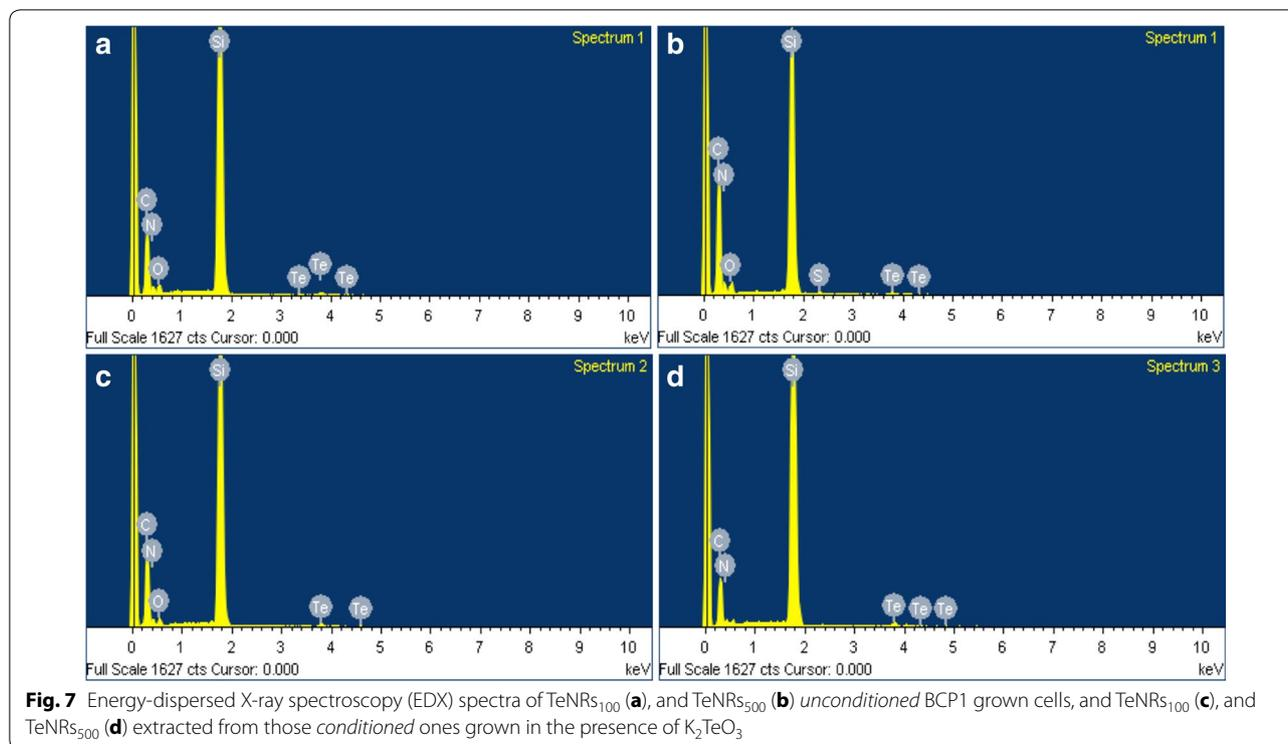
**Fig. 7** Energy-dispersed X-ray spectroscopy (EDX) spectra of TeNRs<sub>100</sub> (a), and TeNRs<sub>500</sub> (b) unconditioned BCP1 grown cells, and TeNRs<sub>100</sub> (c), and TeNRs<sub>500</sub> (d) extracted from those conditioned ones grown in the presence of K<sub>2</sub>TeO<sub>3</sub>
