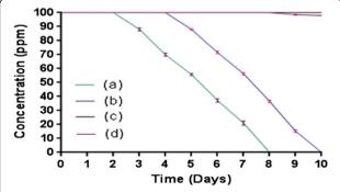
Figure 3 Degradation of 2C4AP by *Arthrobacter* sp. SPG in (a) microcosm with sterile soil, (b) microcosm with non-sterile soil, (c) Un-inoculated control with sterile soil and (d) Un-inoculated control with non-sterile soil.
