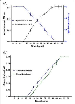
**Figure 1 Growth and degradation studies. (a)** Utilization and degradation of 2-chloro-4-aminophenol by *Arthrobacter* sp. SPG, and **(b)** Estimation of ammonium and chloride ions during the degradation of 2-chloro-4-aminophenol by *Arthrobacter* sp. SPG.
