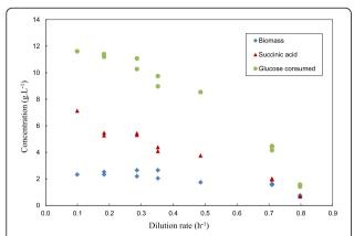
Figure 2 Chemostat steady-state measurements of  $\Delta Glc$ , SA and biomass plotted against D. High shear conditions prevented biomass attachment. Extrapolation of data indicates that  $\mu_{max}$  lies between 0.8 h<sup>-1</sup> and 0.85 h<sup>-1</sup>.
