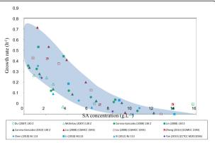
Figure 1 Growth rates vs.  $C_{SA}$  of prominent batch studies on A. succinogenes employing Glc as substrate [12,18-27]. The  $\mu$  values were estimated from the reported biomass/SA vs. time profiles. Severe product inhibition is evident with growth ceasing between 8 g.L $^{-1}$  and 14 g.L $^{-1}$  of SA. The blue data cloud covers the majority of the experimental measurements.
