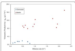
Figure 6 Chemostat and biofilm volumetric productivities  $(q_{SA})$  plotted against D. The comparative  $q_{SA}$  values for the chemostat and biofilm reactors indicate the order of magnitude difference in volumetric productivity. Differences can be attributed to total biomass quantities (see Table 1 and Table 2).
