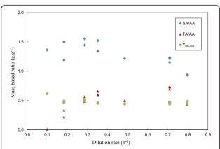
**Figure 3** Chemostat mass-based yield ratios (SA/AA, FA/AA and  $Y_{Glc,SA}$ ) plotted against D. The average  $Y_{Glc,SA}$  is relatively stable at 0.48  $\pm$  0.047 g.g<sup>-1</sup>. FA/AA is close to the equimolar value (0.77 g.g<sup>-1</sup>) at a D of 0.8 h<sup>-1</sup>, decreasing to zero as D is decreased. SA/AA is in the vicinity of 1.4 g.g<sup>-1</sup> for D values below 0.5 h<sup>-1</sup>, while a slight decrease is observed at higher D values.
