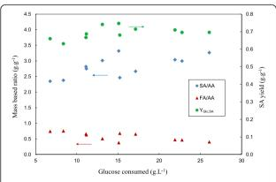
**Figure 7 Biofilm reactor mass-based yield ratios (SA/AA, FA/AA and Y**<sub>Glc,SA</sub>) **plotted against ΔGlc.** When compared to the comparative graph for the chemostat (Figure 3), the Y<sub>Glc,SA</sub> is significantly higher (up to 50% more). The SA/AA ratio of the biofilm runs is more than double that of the chemostat runs (Figure 3). The FA/AA ratio is close to equimolar (0.77 g.g $^{-1}$ ) at low  $\Delta$ Glc but decreases with increasing  $\Delta$ Glc.
