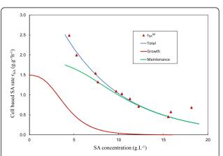
**Figure 8 Breakdown of SA production rate** ( $r_{SA}$ ). Measured total rates are given by the red triangles with the empirical fit given by equation (3). The growth contribution to rate is given by the red curve - obtained from the product of the growth function (equation (2)) and  $Y_{xSA}$  frue (Figure 4). The maintenance contribution to rate is given by the green curve - obtained by subtracting the growth contribution from the total rate.
