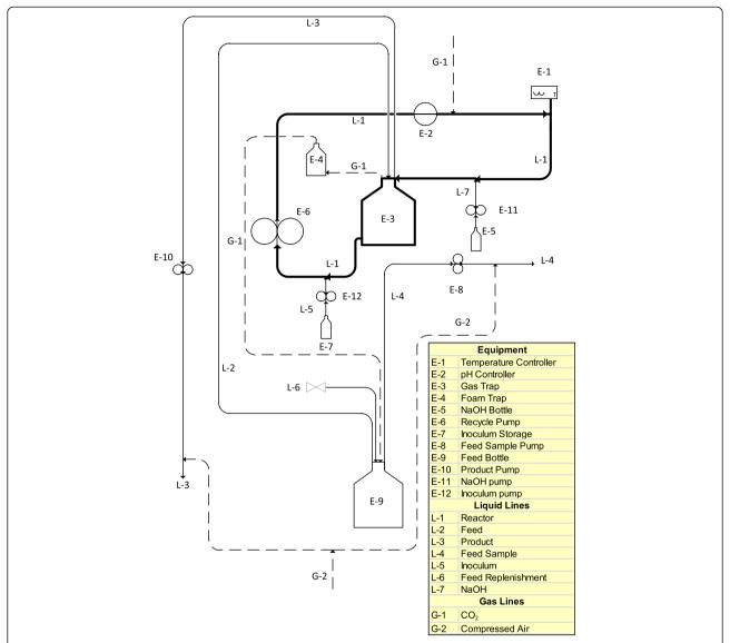
**Figure 9** The bioreactor setup used for both the chemostat and biofilm experiments. The reactor section is shown in bold with an in-line gas trap. The reactor section consists of a 3 mm silicone tube (approximately 5 m length) with an active volume of 50–60 mL, depending on the liquid level in the gas trap.
