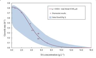
Figure 5 Chemostat growth rates ( $\mu$ ) plotted against SA concentration. Good agreement with the data cloud in Figure 1 is obtained. Inhibition model given by equation (2) with  $\mu_{max}$  at 0.82  $h^{-1}$
