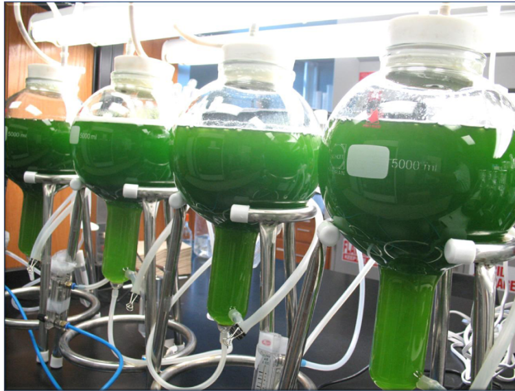
Figure 4 Biomass production of S. bacillaris strain siva2011 in 5 L balloon type bioreactors (working volume 4 L).
