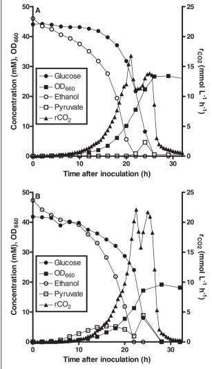
Figure 3 Growth profile of IMI078 (A; Pdc<sup>-</sup> MTH1- $\Delta$ T) and IMI083 (B; evolved Pdc<sup>-</sup>) on high concentrations of glucose. Cultivation in an aerated pH-controlled (pH 5) bioreactor with 7.5 g Γ<sup>-1</sup> glucose and 0.3% (v/v) ethanol. The results are from one representative experiment. Duplicate experiments deviated <5% in titers, CO<sub>2</sub> production and OD<sub>660</sub>.
