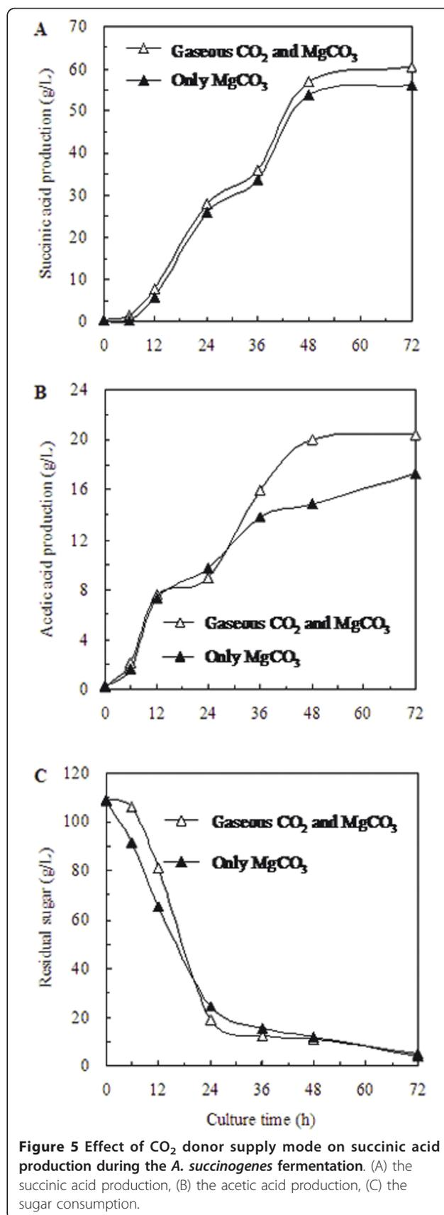
**Figure 5** Effect of  $\text{CO}_2$  donor supply mode on succinic acid production during the *A. succinogenes* fermentation. (A) the succinic acid production, (B) the acetic acid production, (C) the sugar consumption.
