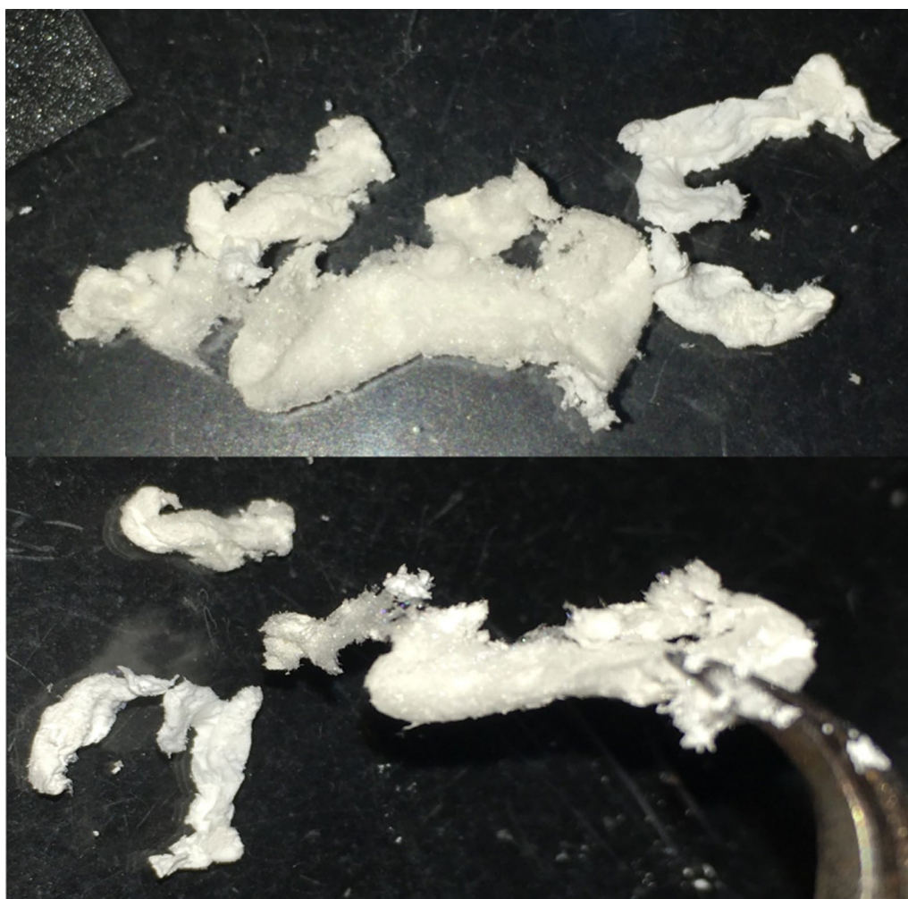
Fig. 7 Purified A5 4mer spider silk protein produced through the microbial conversion of depolymerized polyethylene. The silk protein was dialyzed into water and lyophilized, resulting in several discrete and cohesive chunks of a white, polymeric material that ranged in length from approximately 1.5–4 cm. This image was obtained directly after the freeze-drying process, and the protein sample had not been spun into fibers or put through any additional material processing
