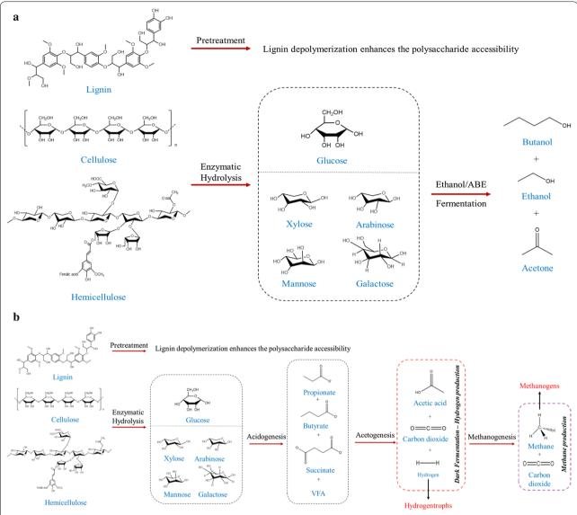
Fig. 5 a Schematic representation of fermentation strategy adapted for second generation alcohol production. b Schematic view of the anaerobic digestion strategy for LCB conversion into biohydrogeand biomethane
