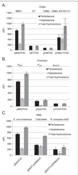
Figure 2 Hydrocarbon titers for the various (A) origins of replication, (B) promoters, and (C) RBS sequences; (dark bars) pentadecane, (light bars) heptadecene, and (grey bars) combined.
