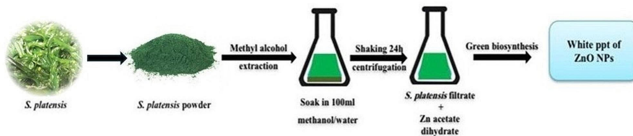
Fig. 1 Schematic illustration of the sustainable green synthesis of ZnO NPs
